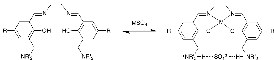
Scheme 3. Expected binding of metal sulphates with salen-based zwitterionic receptors.
